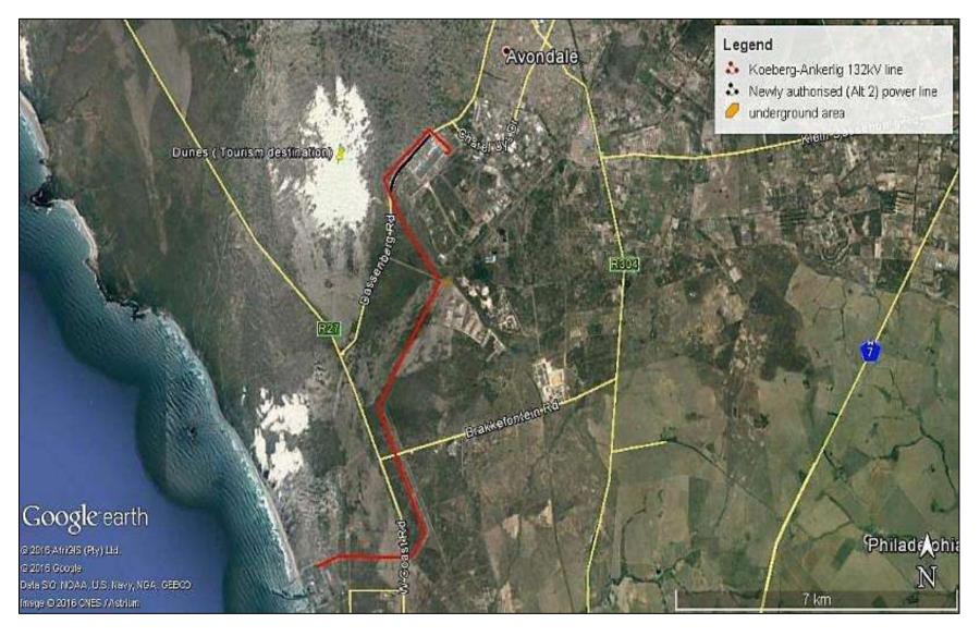
**Figure 1:** The newly authorized (Alternative 2) power line (black line) from the Atlantis substation and the Koeberg power line (red line) are depicted here. It is ~14 km from Ankerlig Power Station to the Koeberg Power Station.
